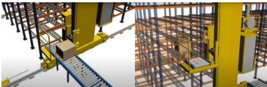
Gambar 3. Automated Storage and Retrieval System (AS/RS) dengan Aisle-Captive Cranes
